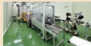
Automatic Packaging Line & Palletizer
